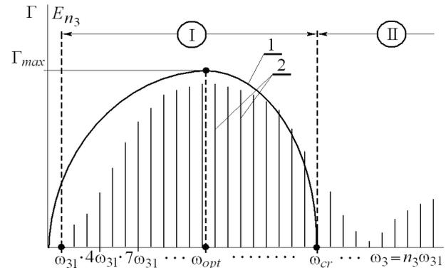
**Fig. 6** – Dependence of the increment of SCW rise (curve 1) on the SCW frequency, and typical for cluster FEL spectrum 2 of higher SCW harmonics in two-stream high-current relativistic beam
