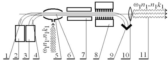
**Fig. 3** – Structural scheme of two-stream cluster FEL-klystron with non-resonant modulator 5 and multiharmonic (cluster) input signal
