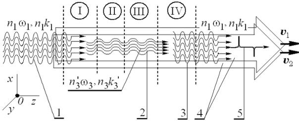
**Fig. 5** – Generalized theoretical model of two-stream cluster FEL-klystron for the devices shown in Fig. 1-Fig. 4
